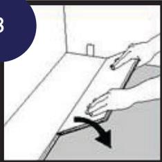
Place first plank of the new row with the tongue side at an angle against the groove side of the plank in the previous row. Press forward and lay it flat at the same time.
