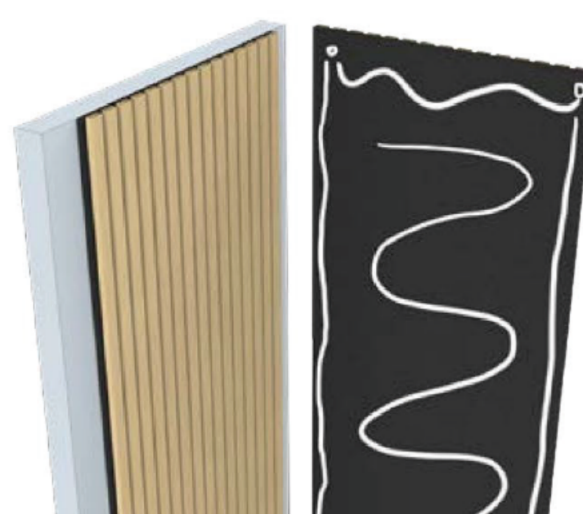
b. Attach acoustic panels to the wall with nail-free glue. absorption class: D
